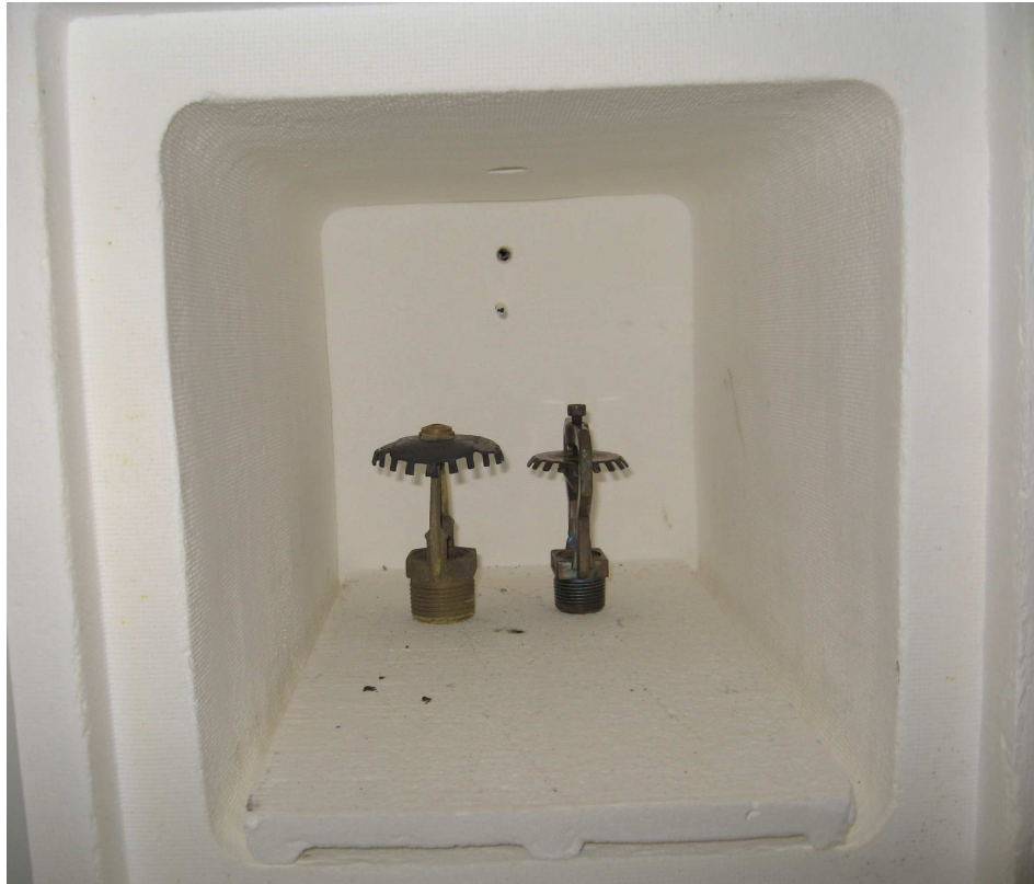
Figure 10 Heat Resistance Samples – Test Set-Up
