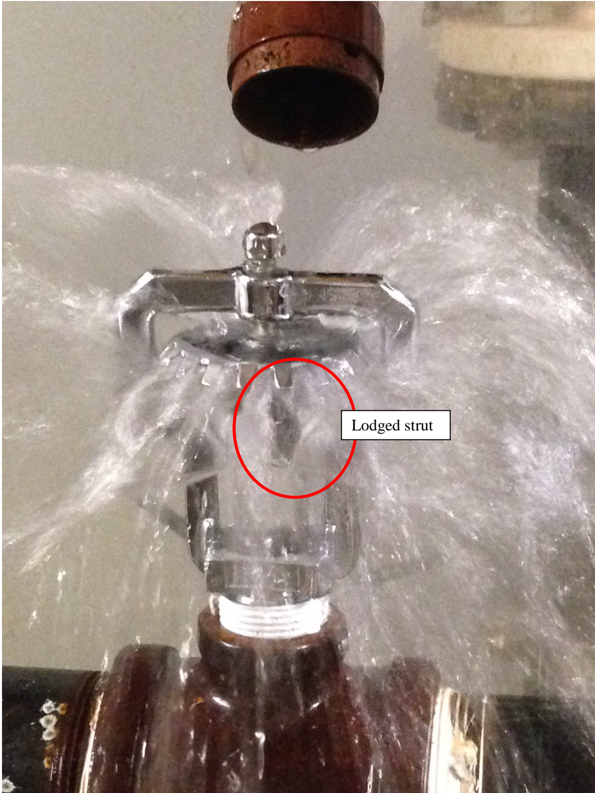
Figure 8 ESFR-202, Non-compliant Lodgment Test
