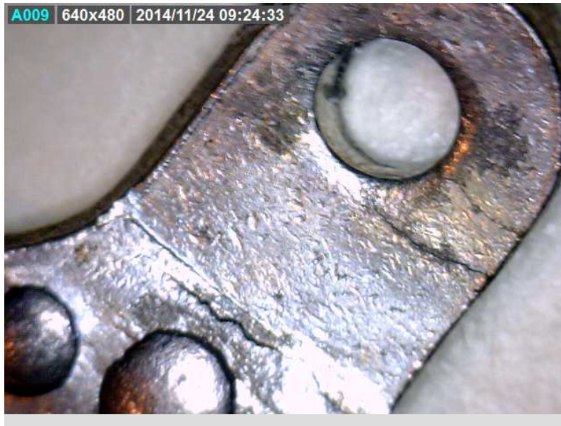
Figure 16 ESFR-202 Lever – Images of Post-Stress Corrosion Cracking of Stainless Steel Parts Test
