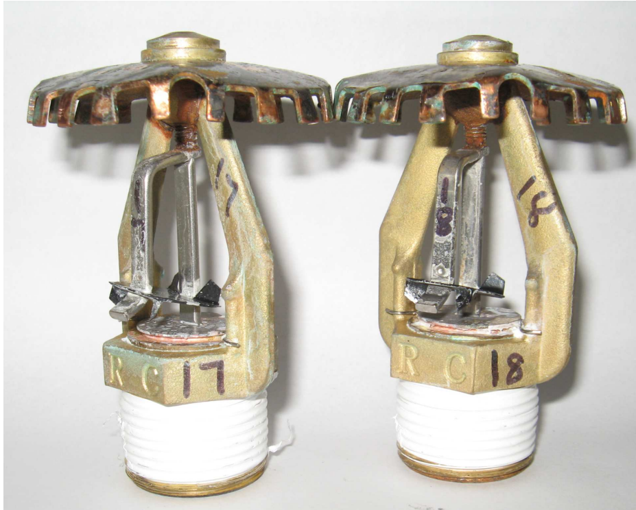
Figure 13 ESFR-363 10-Day Corrosion Samples, Post-Sensitivity Test
