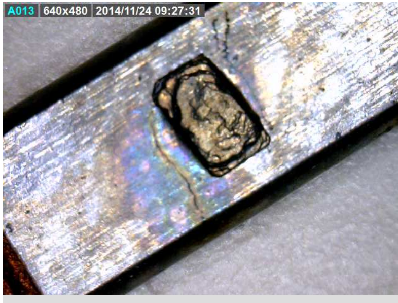
Figure 15 ESFR-363 Strut – Images of Post-Stress Corrosion Cracking of Stainless Steel Parts Test
