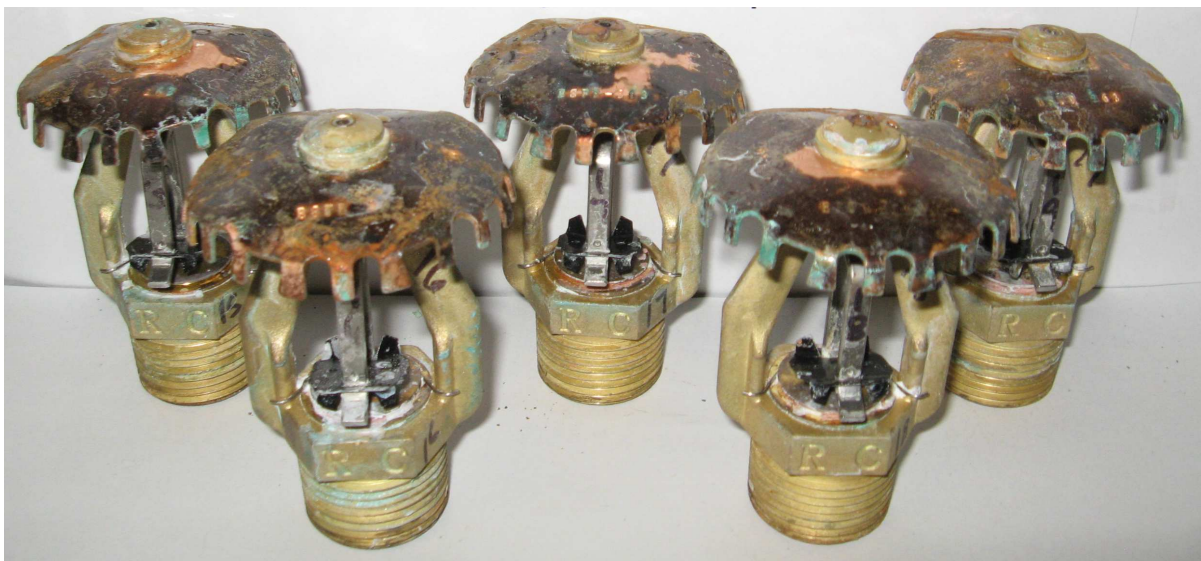
Figure 12 ESFR-363 Post-10-Day Salt Spray Exposure
