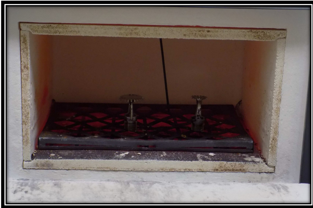
Figure 15 Heat Resistance Samples – Test Set Up
