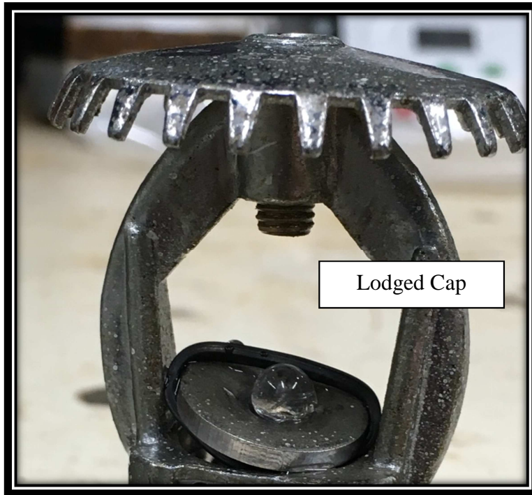
Figure 13 Sample U89 – Double Feed Upright, Non-compliant Lodgment Test
