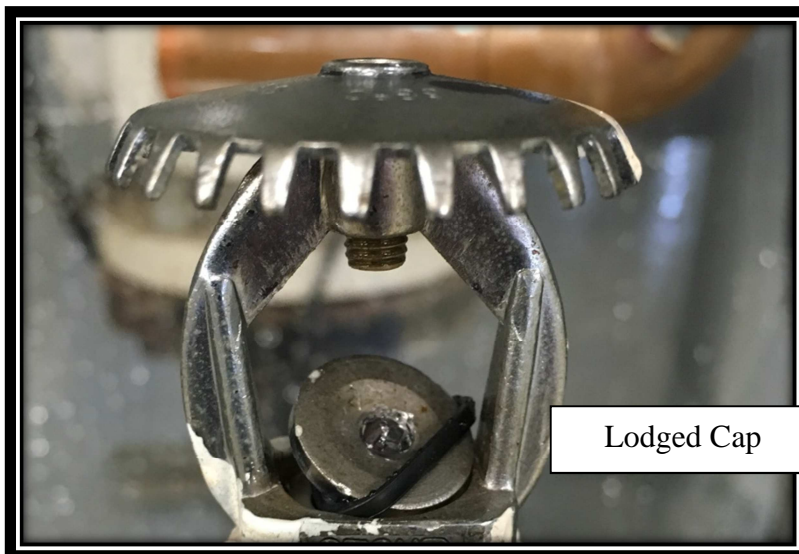
Figure 14 Sample U98 – Double Feed Upright, Non-compliant Lodgment Test
