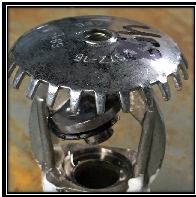
Figure 9 Sample U58 – Single Feed Upright, Non-compliant Lodgment Test
