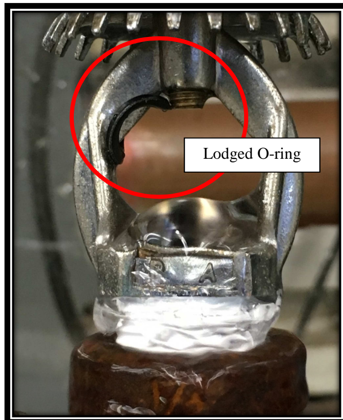
Figure 12 Sample U74 – Double Feed Upright, Non-compliant Lodgment Test
