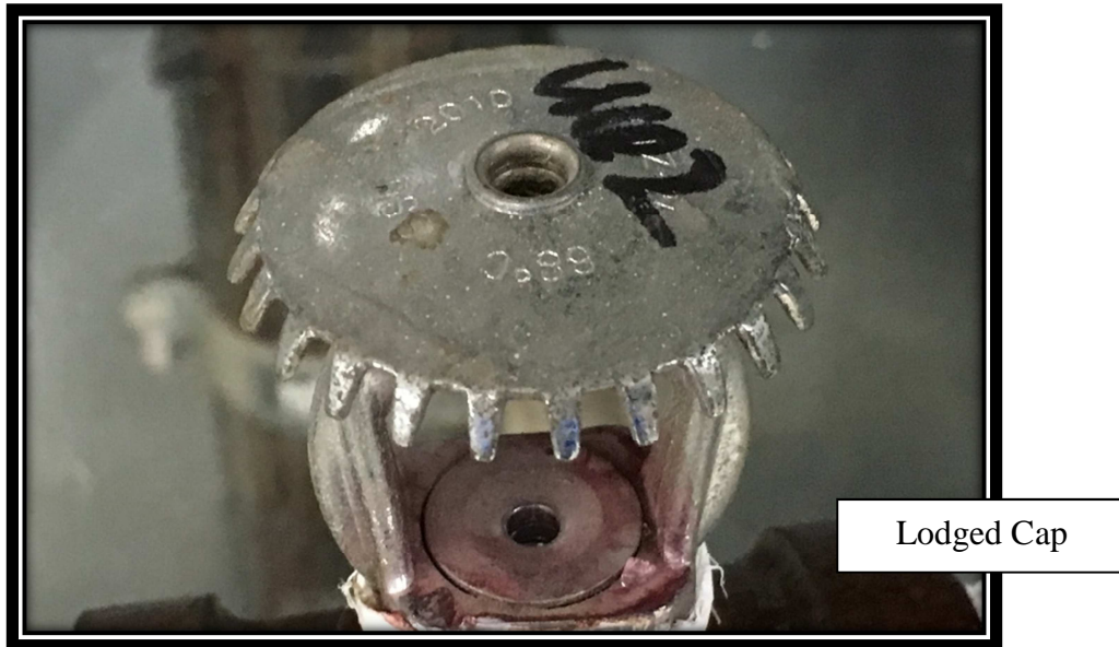
Figure 11 Sample U62 – Double Feed Upright, Non-compliant Lodgment Test
